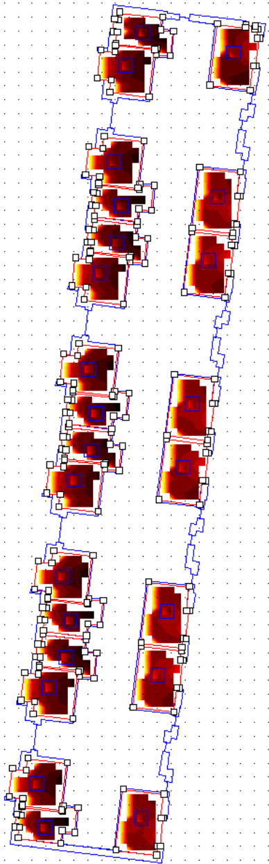
Figure 117 - Duplex Block 3 Second Floor Daylight Factor Mapping
