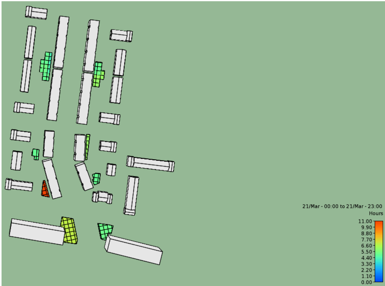
Figure 7 – Sunlight to Amenity Areas (Northern section) – More than 50% > 2 hours (Source IES VE Suncast)
